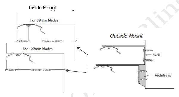
Position the brackets so that the blades clear the window frame or any protruding handles.
